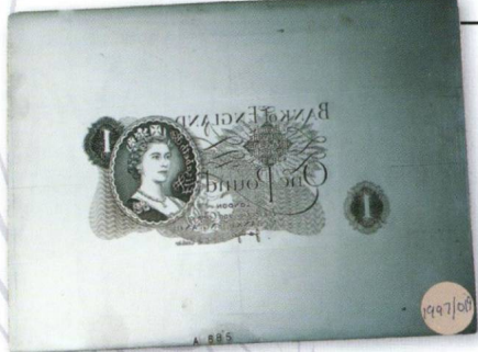
Above: Steel Master die for the Series C £1 banknote of 1960, showing in reverse the portrait featured on one of the new Jubilee definitives
